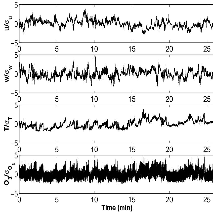
Time series of simultaneously measured turbulent velocity components, air temperature, and ozone concentration. For comparison purposes, we normalized all the time series measurements to zero-mean and unit variance.
