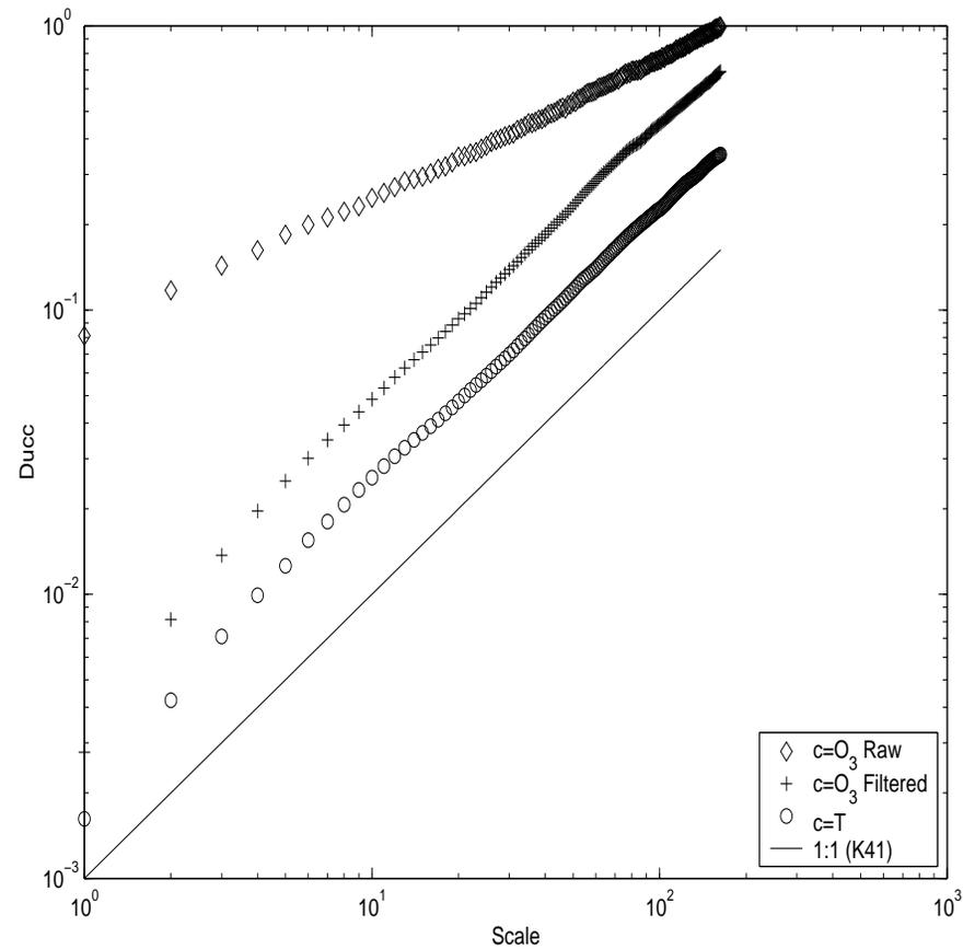
Computed mixed structure functions ( $D_{u'CC}$ ) for  $C$  representing filtered and raw  $O_3$  time series with  $u'$ . For reference, the mixed structure function between  $T$  and  $u'$  is also shown along with  $\tau^1$  from **K41**.
