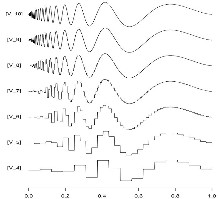
Left: Multiresolution Analysis of doppler function. The original function in  $V_{10}$  is a sum of projections on  $V_4$  and  $W_4$ – $W_9$  subspaces. Right: Coarsening doppler function by projecting it to  $V$ -subspaces.
