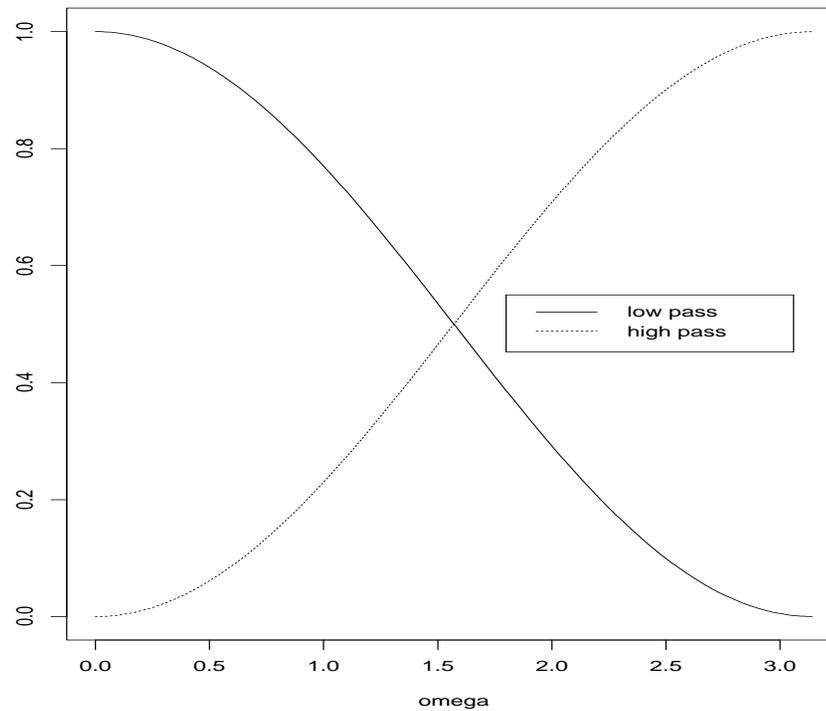
Functions  $|m_0(\omega)|^2 = \cos^2 \frac{\omega}{2}$  and  $|m_1(\omega)|^2 = \sin^2 \frac{\omega}{2}$  for the Haar case.
