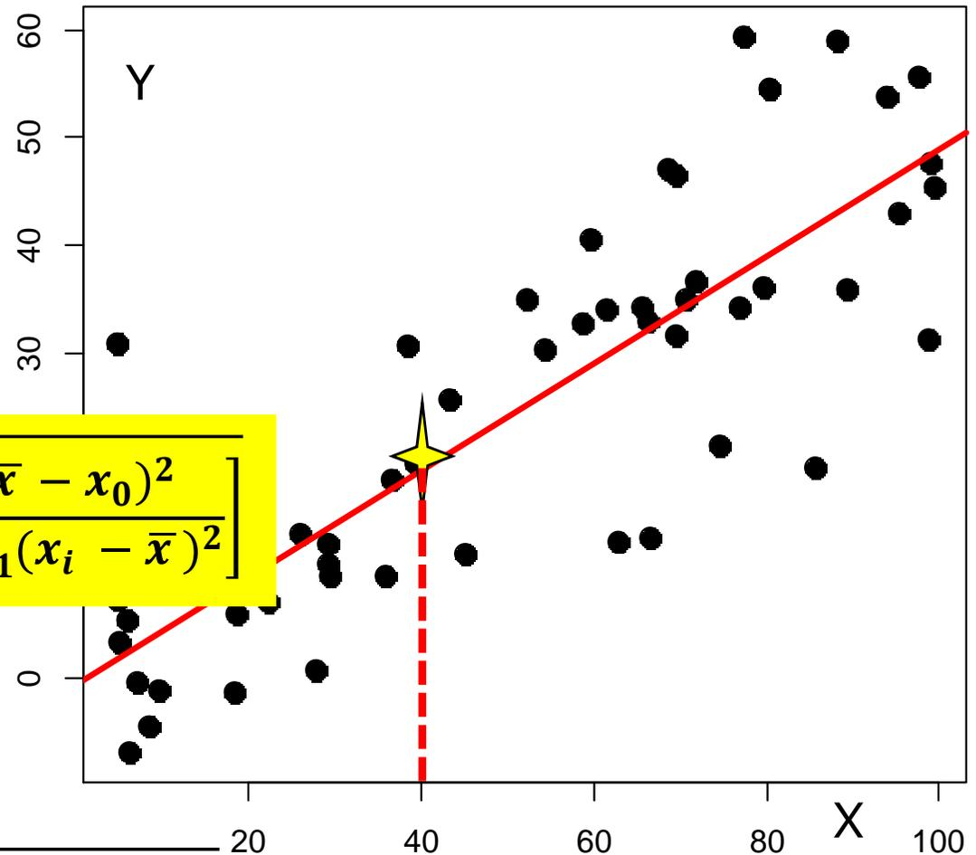
$$\hat{y}_0 \mp t(n-2)_{\alpha/2} \times \sqrt{s^2 \left[ 1 + n^{-1} + \frac{(\bar{x} - x_0)^2}{\sum_{i=1}^n (x_i - \bar{x})^2} \right]}$$
